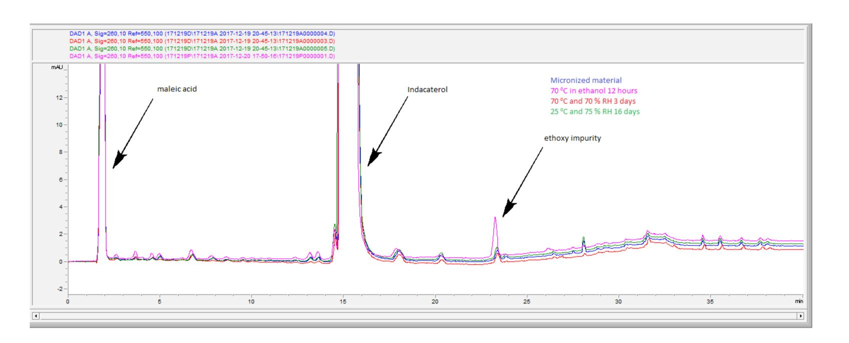
HPLC chromatograms of micronized IM before Figure 1 and after annealing at different conditions.
