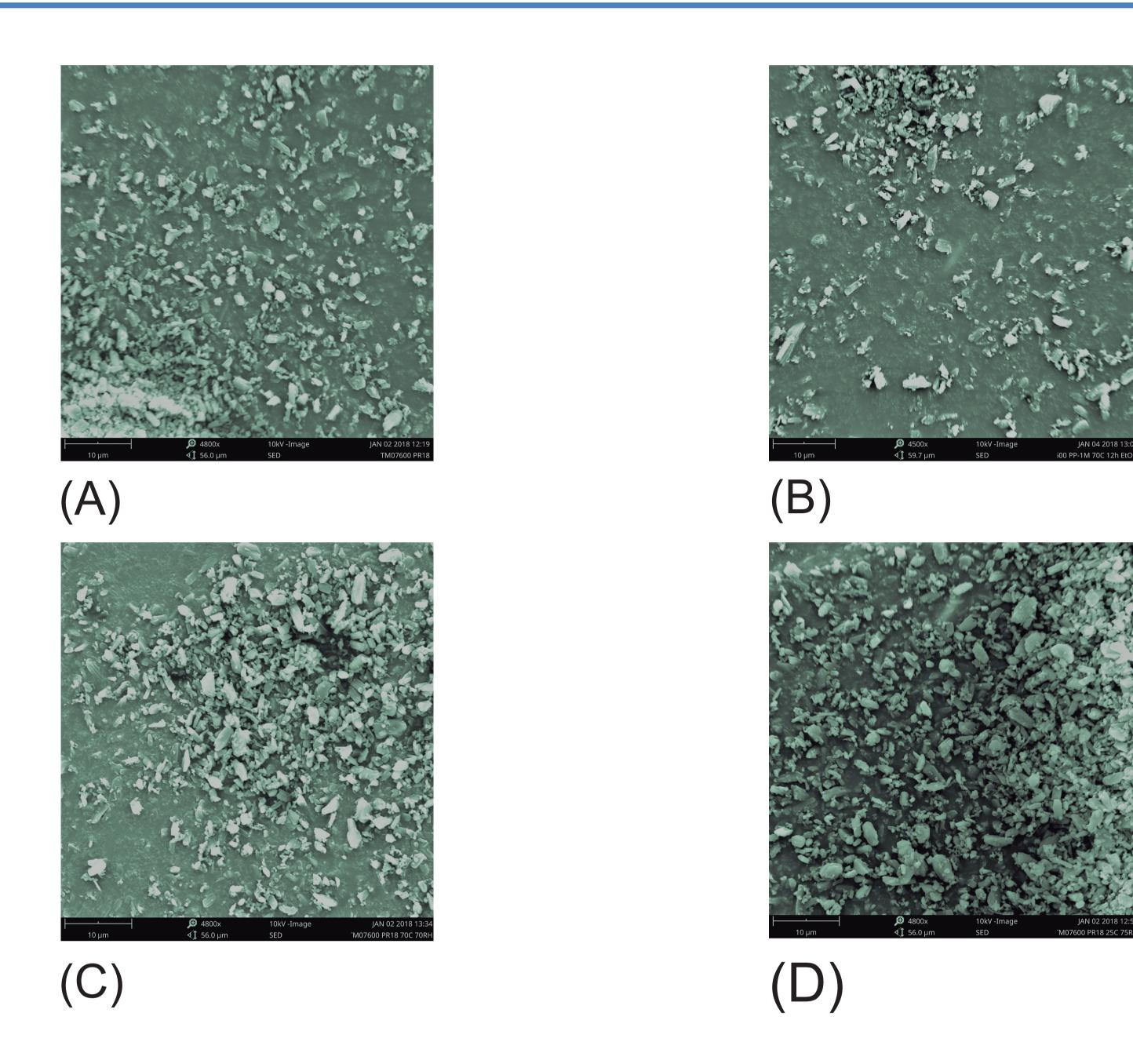
Figure 3 - SEM image of (A) freshly micronized IM, (B) annealed IM at 70°C in ethanol (C) annealed IM at 70°C and 70% RH and (D) annealed IM at 25°C and 75% RH.
